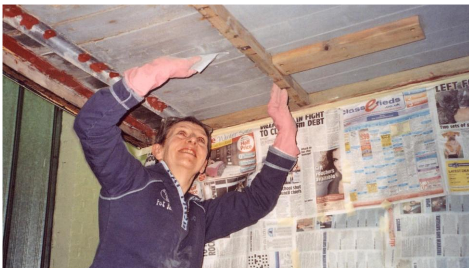
June Corney preparing the underside of the upper saloon floorboards for painting, March 2011
